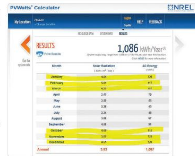
This highlighted data shows the solar gain striking a south wall in winter in Denver, Colorado.
