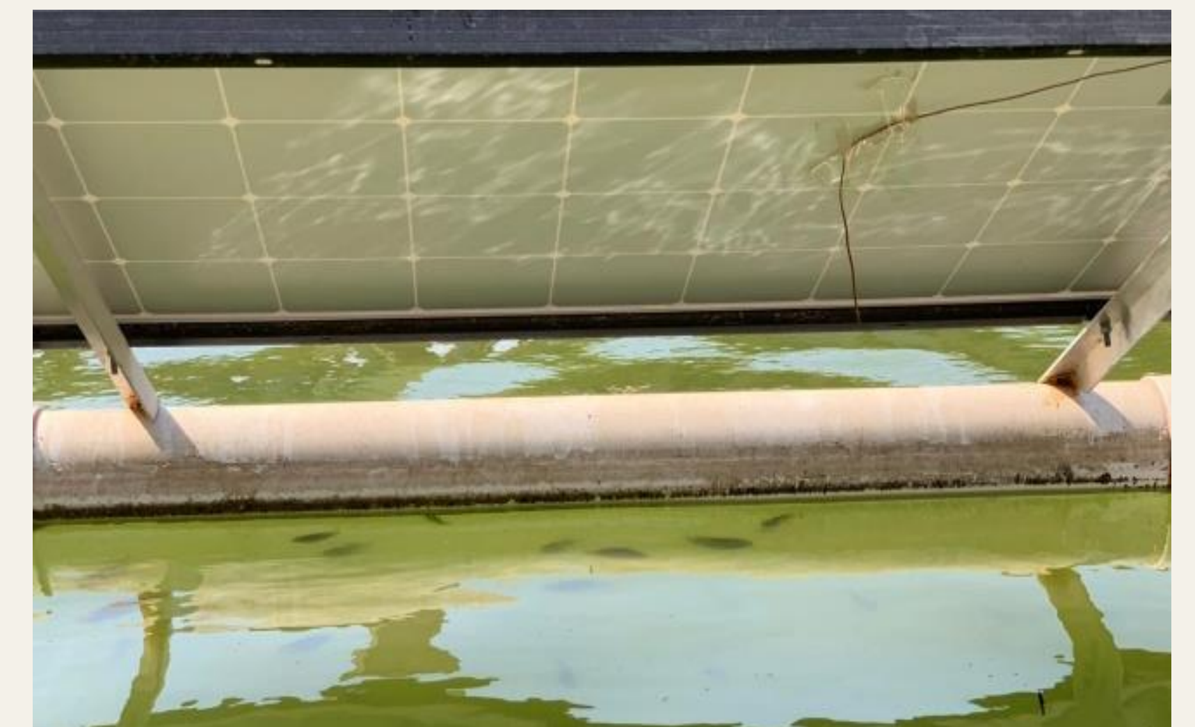
Fig. 9. Sun light reflection on the back surface of the solar panel.
