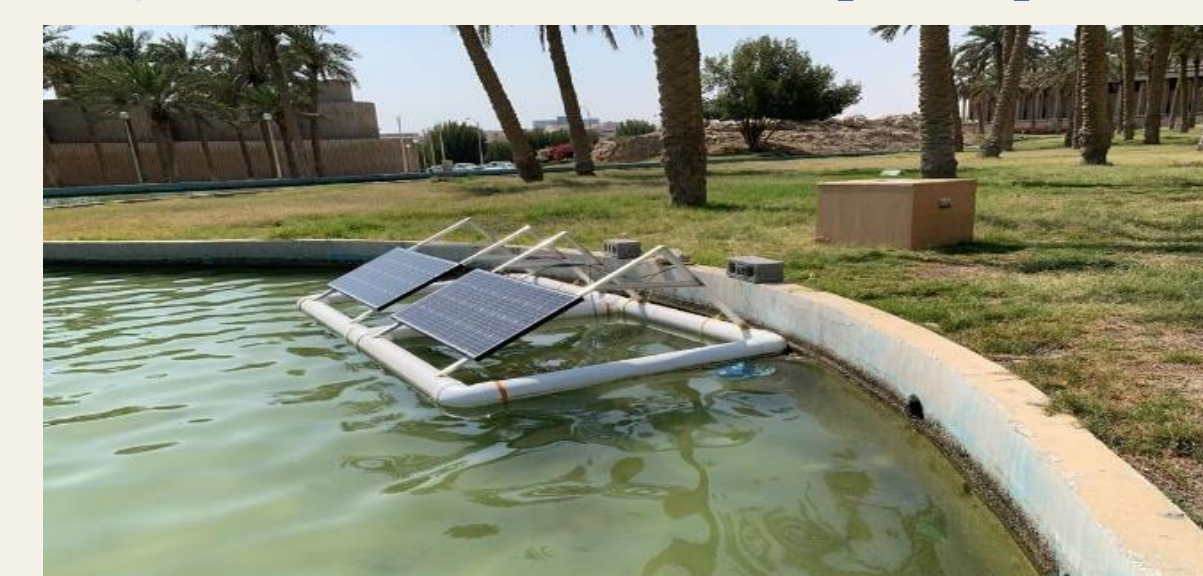
Fig. 5. Experimental set up of the FPV assembled in-house
