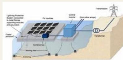
Fig. 4. Schematics of an FPV power plant [8].
