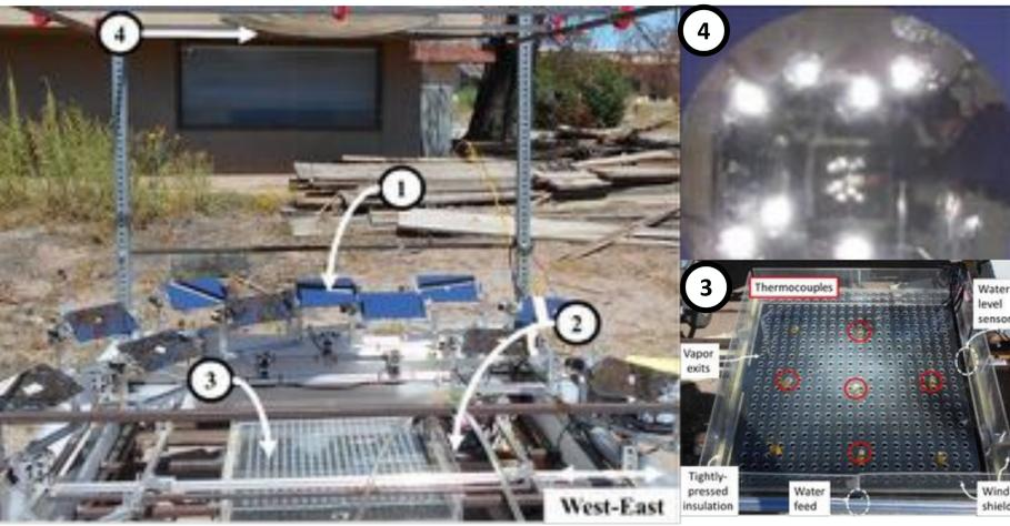
**Figure 1.** Main components of the experimental setup. 1) Heliostat field distribution, 2) Water level controller, 3) Polycarbonate basin and 4) circular hyperbolic central mirror (for the BDC configuration).
