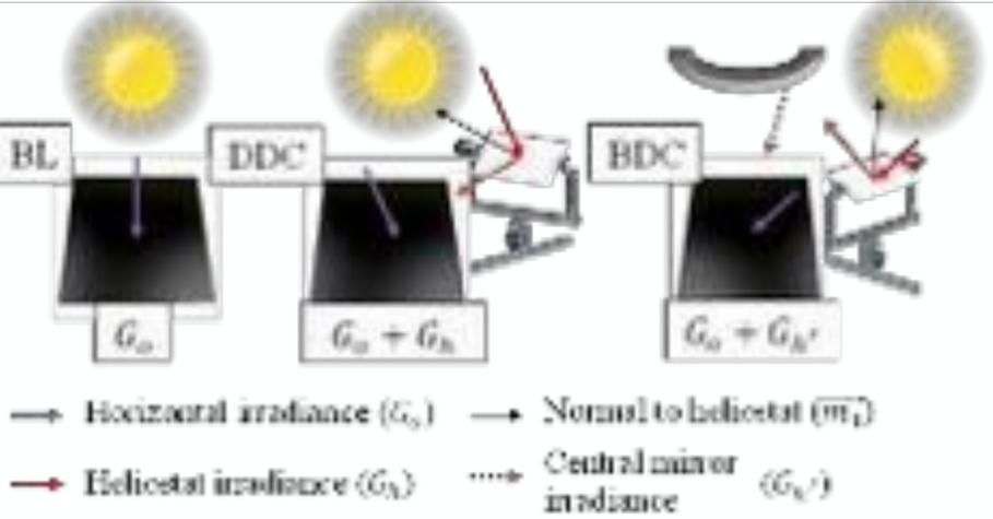
**Figure 2.** Different configurations tested for water desalination.
