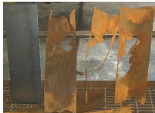
Fig 7. New and Depleted EC TM Electrodes
