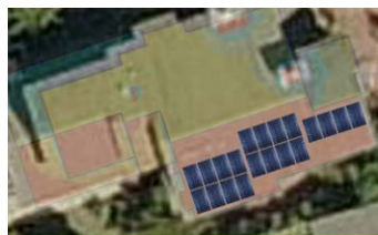
Figure 6: Outline of the building, color coded solar potential and module placement on the roof.
