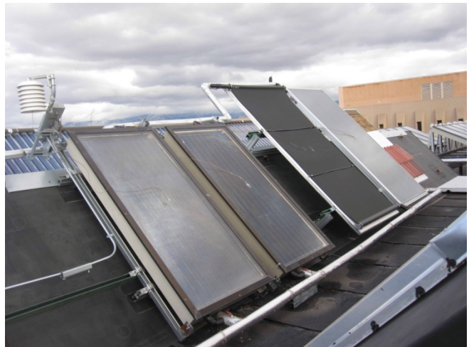
Photo 2. Four different collector types that can operate with UNM's Solar Hot Water Reliability Testbed.
